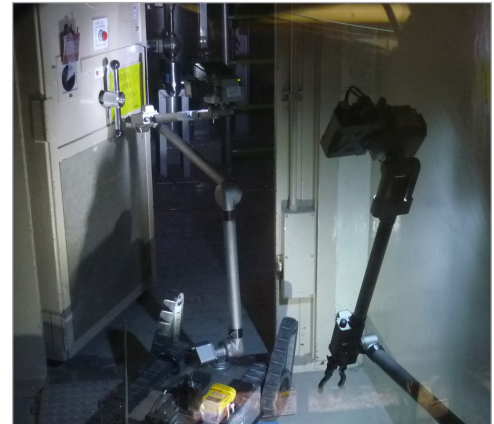
PackBot supports multiple sensors including thermal camera and sensors for HAZMAT and radiation detection.
