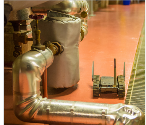
At just 4.9" H X 9" W X 10.3" L, FirstLook has cameras on all four sides, making it a good fit for inspection.
