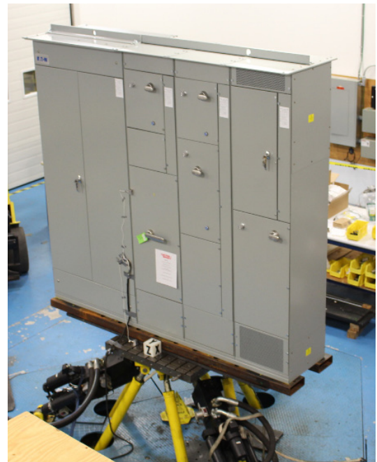
MCC (2.5m x 0.5m x 2.2m) Being Seismically Qualified In-House
