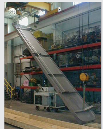
Transfer Canal Pool Gate
