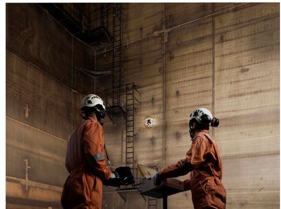
The lightweight, confined-spaces drone not only flies, but also rolls lightly and easily over obstacles.
