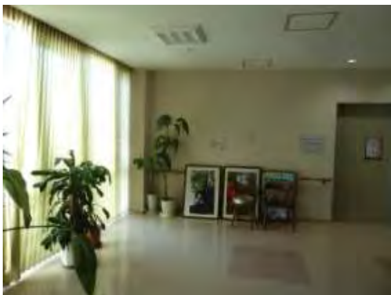
Out of concern for further aftershocks, the hospital placed art and other wall mounted objects on the floor (left). Heavy furniture that can overturn, such as the tall cabinet on the right, were also lowered to the floor so that they would not tip over in aftershocks. I have visited many hospitals, and other public buildings along the Pacific West Coast and throughout the world after earthquakes – this thoughtful precaution was a first for me.
