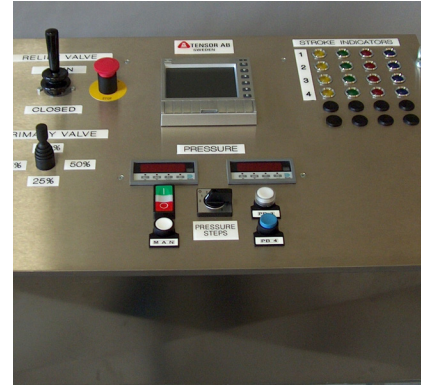
Each bolt tensioner is equipped with an 'easy-to-read' stroke indicator box that provides the pump operator with the condition of its stroke using yellow, green, red, and blue indicating lights.
